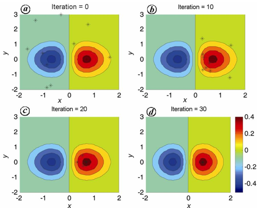
**Figure 5.** Illustration of the working of the PSO algorithm, showing over the iterations how the particles explore the global optima. The colour scheme gives the quality of fitness value (objective value). Blue colour corresponds to minimum  $f$ , whereas dark red to maximum  $f$ .
