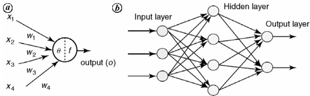
**Figure 7.** Architecture of artificial neural network. *a*, Artificial neuron; *b*, Multilayered feed-forward neural network.
